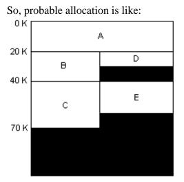
The figure illustrates a storage assignment for each procedure consistent with the overlay structure. This over all scheme is called dynamic binding or load-on-call.
