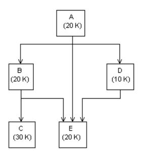
The figure high lights the inter dependencies between procedures. The procedure B and D are never in use at the same time and procedure C and E also. If we load only those procedures that are actually be used at any particular time. The amount of memory needed is equal to the longest path of the overlay structure.
