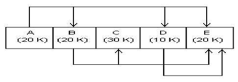
The figure illustrate a program consisting of five subprograms A,B,C,D,E that require 100 bytes of core. The arrow indicates that the subprogram A only calls B, D and E does not call any other subroutines.
