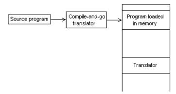
This is also called assemble-and-go loader. It is one of the easiest to implement. Here, the assembler runs in one part of the memory and places the assembled machine code, as they are assembled, directly into the assigned memory locations. So, assembler must always be present in the memory. It has 3 main disadvantages:
