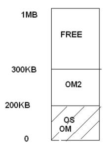
In the main memory, already OS occupies the memory from 0 to 200KB.Now the object module OM has to be placed over the OS from 200KB onwards. But OM has been placed from 0 to 200KB.Now there is an overlap, this leads to problems and confusions. The module OM has to be addressed from 200KB to 400KB.So the starting address of OM is 200.This is called relocation.
