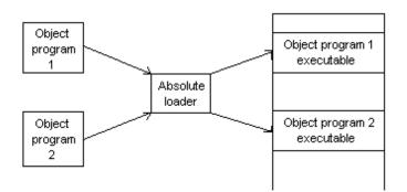
Here, the assembler outputs the machine language translation of the source program in almost the same form as in the 1<sup>st</sup> scheme. But here, the assembler is not in memory at
