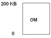
This object module occupies 200KB of memory from 0 to 200KB. This has to be loaded into the main memory.
